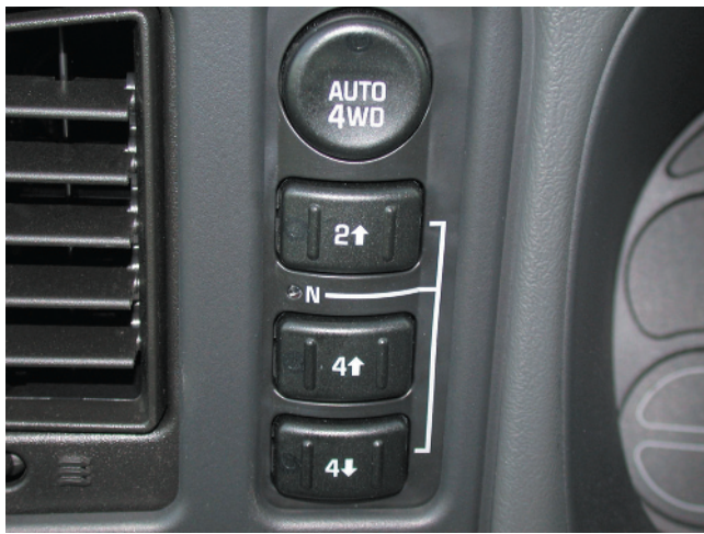
FIGURE 1-9 A dash control panel used by the driver to control the four-wheel-drive system.
