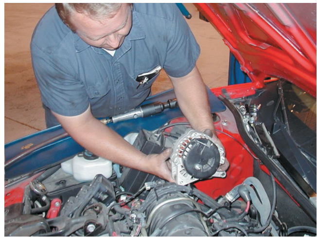
FIGURE 1-10 The alternator is in the heart of the electrical system.
