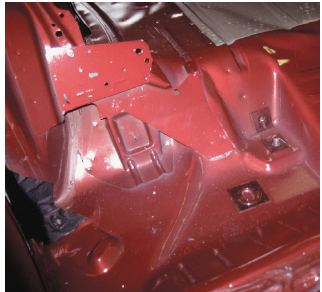
FIGURE 1-5 Note the ribbing and the many different pieces of sheet metal used in the construction of this body.
