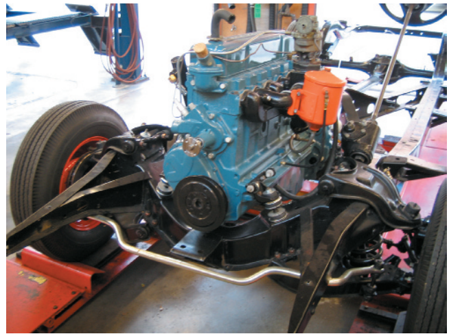
FIGURE 1-3 A chassis of a 1950s era vehicle showing the engine, drivetrain, frame, and suspension.
