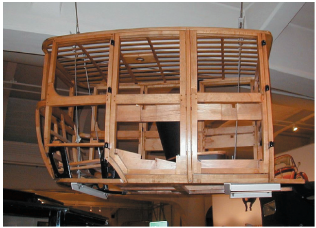
FIGURE 1-2 Most vehicle bodies were constructed with a wood framework until the 1920s.
