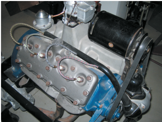
FIGURE 1-7 A Ford flathead V-8 engine. This engine design was used by Ford Motor Company from 1932 through 1953. In a flat-head design, the valves located next to (beside) the cylinders.
