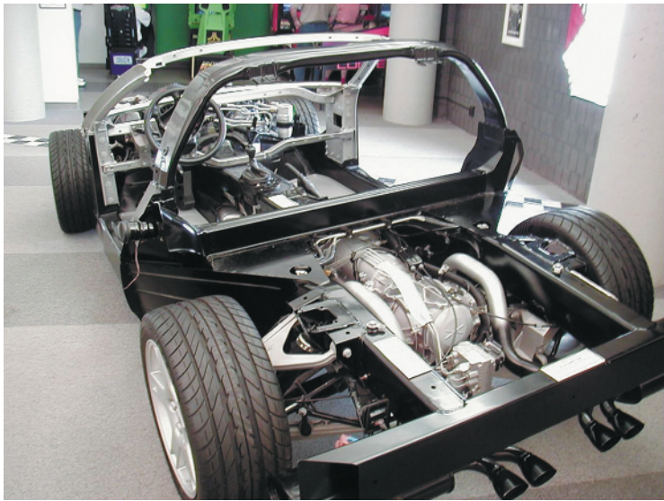
FIGURE 1-6 A Corvette without the body. Notice that the vehicle is complete enough to be driven. This photo was taken at the Corvette Museum in Bowling Green, Kentucky.
